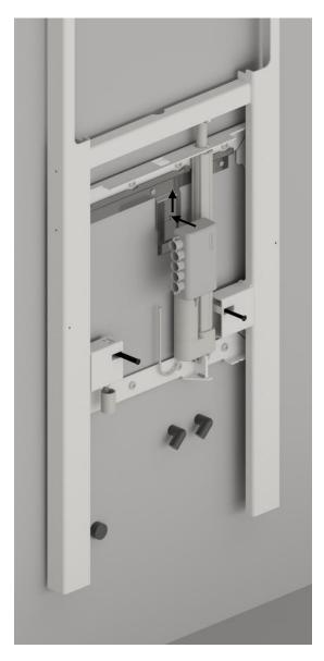
Mount the control box on the mounting bracket. Make sure that the small aluminum leg interlocks and locks the box in a fixed position.
