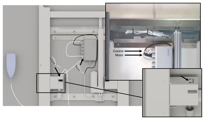
If no fixed control has been chosen, mount the control with cable in the control box as shown. Fix the excess cable from the power supply on the mounting bracket with strips. Check that the unit freely moves up/down. If needed, use cable clips etc. for the power cable.
