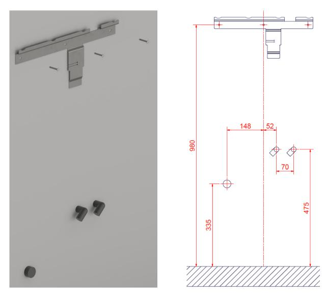
Fix the mounting bracket as illustrated on the drawing with the right distance to water and drain. Make sure that the mounting bracket is level.
