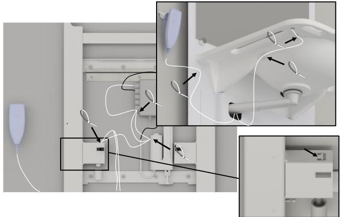
For the fixed control, it's recommended to lead the cables and fix them as shown, after the covers and washbasin has been mounted. The control cables are fixed to the mounted cable holders.
