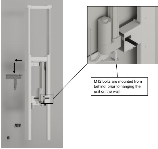
Hang the lifting unit on the mounting bracket. **Make sure** to put the M12 bolts for the washbasin in the frame prior to mounting.
