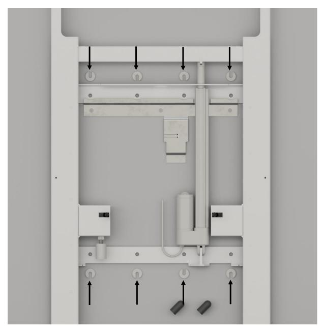
Push 8 spacers in behind the frame so that it has the right distance to the wall. Mark the 8 holes for fastening. Take the lifting unit down again and drill the holes in the wall.
