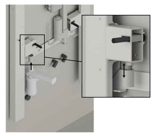
Install the siphon. Adjust the holder bracket according to the washbasin to be mounted. The height of the bracket depends on the height of the washbasin.
