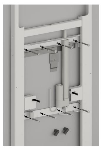
Use suitable rawlplugs and screws for the mounting.
