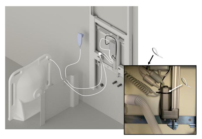
If the fixed control has been purchased as an accessory, mount the Y-cable in the control box, then lead the wires as shown. The wires should be pulled through the outer cover, for the best possible wiring. Fix the excess cable from the power supply on the mounting bracket with strips.
