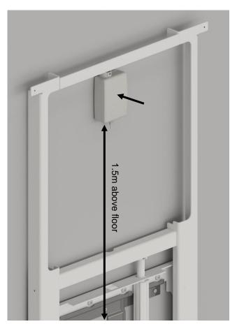
Remove the protective foil on the tape and fasten the power supply above the unit. Place it 1.5 m above the floor measured to the underside. Place it in the middle of the lifting unit.
