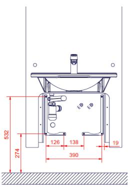
Alternatively, the brackets can be screwed to the wall. Use the shown measurements (mm).
